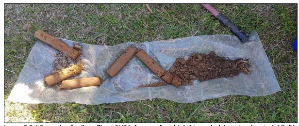
Image 7.2.1 Example of soil profile at BH04, from surface (right) to underlain natural material (left)
